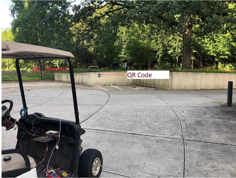
Figure 6-5: Setup to validate the docking procedure
