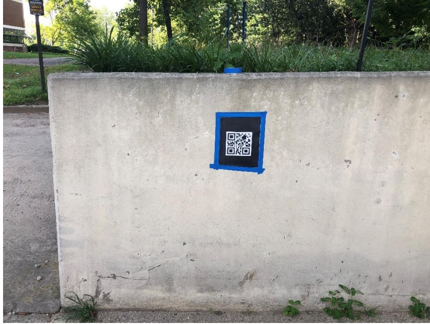
Figure 6-6: QR code mounted on the wall serving as a visual marker
