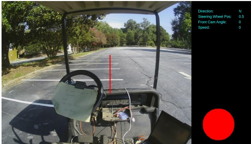
Figure 3-13: Snapshot of GUI at the operator station
