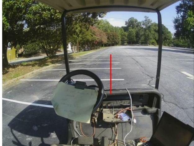
Figure 4-16: An example image with steering guidelines overlaid on the image being transmitted to the operator
