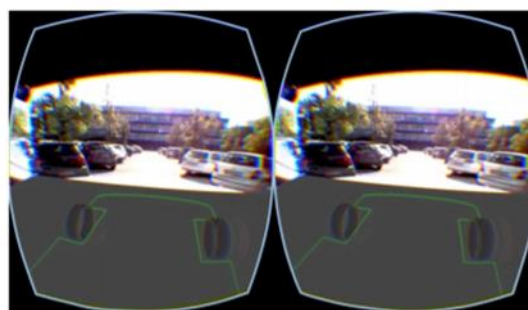
Figure 2-7: Teleoperated driving within a narrow passage using visualization of the remote vehicle in the virtual environment (Hosseini & Lienkamp, 2016)
