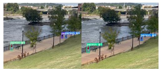
Figure 16: Example of occlusion with the DeepSort tracking on the Columbus RiverWalk
