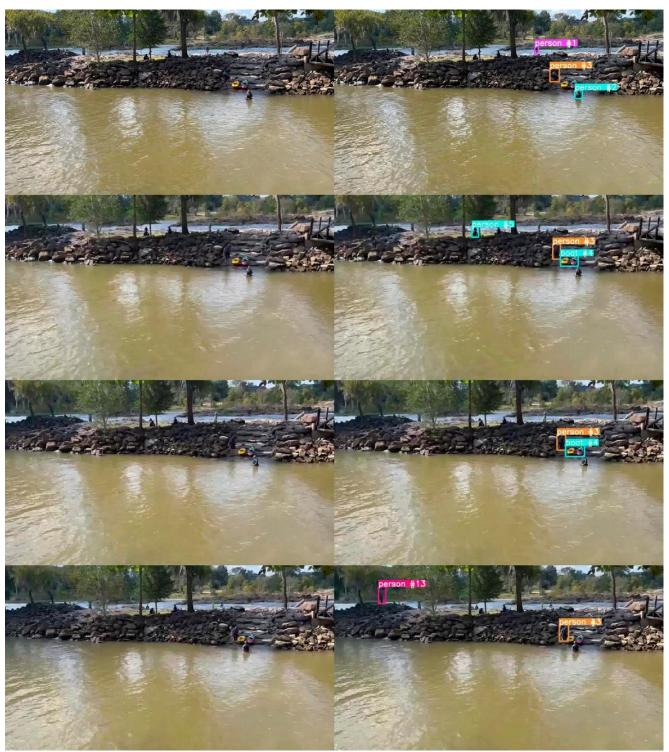
Figure 21: YOLOv5 applied to profile view of rock island near 14<sup>th</sup> street
