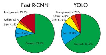
Figure 5: A comparative breakdown of YOLO and Fast R-CNN
