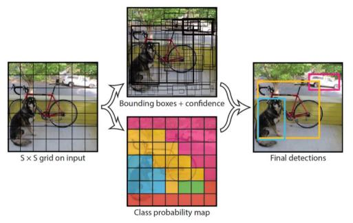
Figure 9: YOLO three step object detection process
