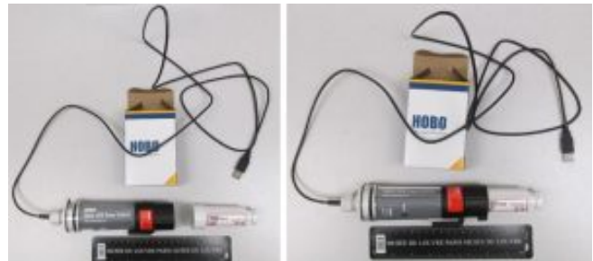
Figure 38: HOBO Data recording system using HOBO Basze U-4. Universal Optic USE Base Station and HOBO Pro v2 Temp/RH Logger. System plugs into laptop ( https://www.onsetcomp.com/search/products/HOBO. ) Photo: Larry Barksdale, UNL
