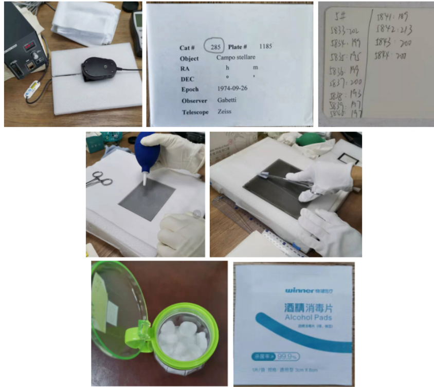
Figure 5: Plate preparation for scanning at SHAO
