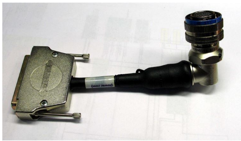
Figure 19 - CCD cryostat video cable
