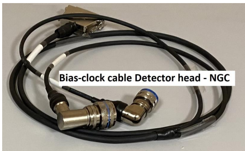
Figure 13 – Detector Cryostat Cables (DCC)
