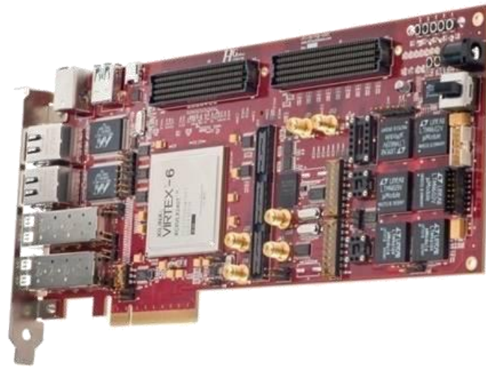
Figure 11 - The PCIe interface board (DAQC)
