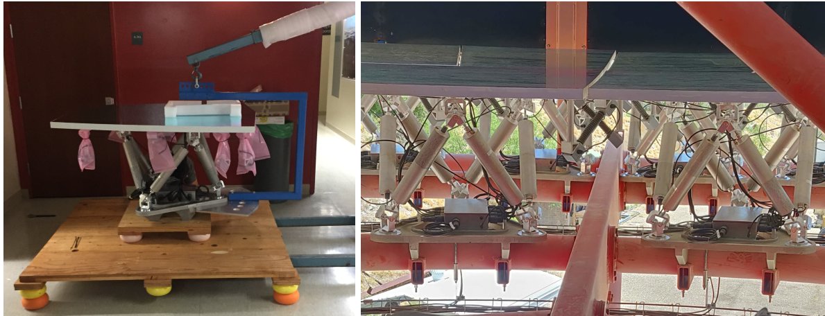
Figure 3. (Left) A P1 panel after assembly and MPES calibration shown during packaging for shipment to FLWO. The panel is lifted with a floor crane, hovering above the base of the shipping crate. The MPES units attached on the back of the mirror panel are covered for protection. Six actuators that form a Stewart platform, a controller board, and the mounting triangle interface to the OSS are visible. A custom-made blue U-shaped jig is attached to the mounting triangle and the floor crane. (Right) Side view of two “sectors” of M1 panels installed on the pSCT. A P1 panel has two P2 neighbors on the outside, forming a so-called “sector”. A “long edge” consisting of a P2-P2 edge and a P1-P1 edge along the azimuthal direction between two “sectors” is visible.
