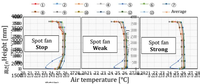
Figure 10. Vertical temperature distribution under  $26^{\circ}\text{C}$  conditions
