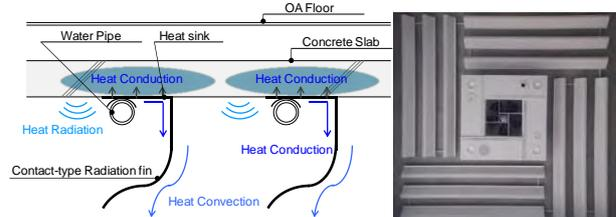
Figure 2. Contact-type radiation fins
