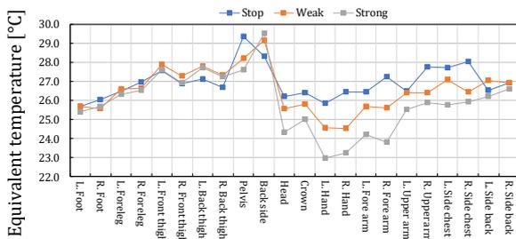
Figure 12. Equivalent temperature on each body segment under  $27^{\circ}\text{C}$  conditions
