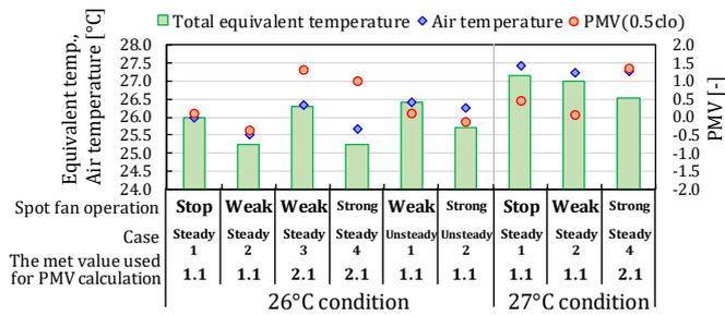
Figure 11. Total equivalent temperature by thermal manikin
