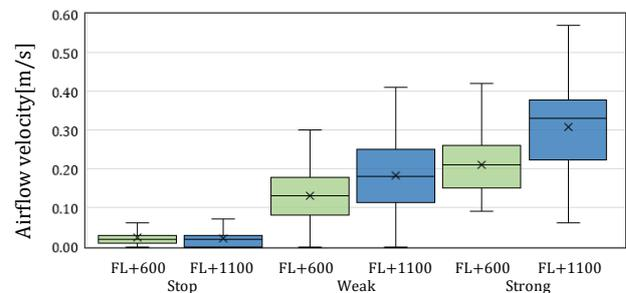
Figure 9. Airflow velocity during subject experiments
