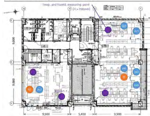
Figure 6. Layout of the TCC users (f1, f2: female, m1-m6: male)
