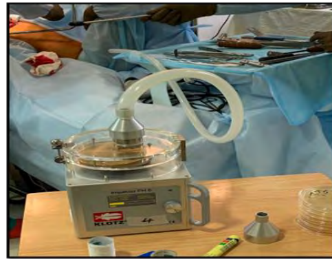
Figure 11: Klotz Impactor FH6 for active air sampling
