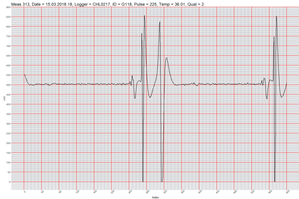
Figure S4. Example of an ECG signal (quality level 2) with incorrect estimation by the internal algorithm (225 bpm) and the manual validation (6.6 red squares between two R-waves = 34 bpm), typically resulting from double counts of one ECG cycle.
