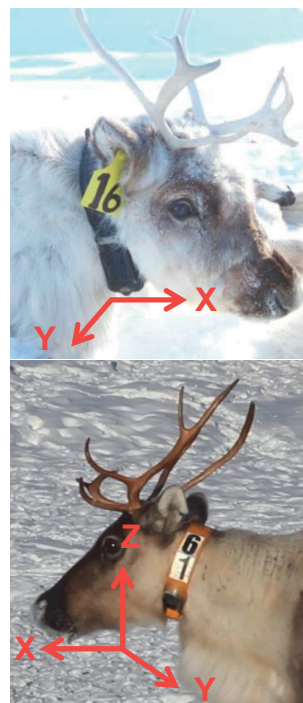
Activity sensors and axes recorded. Top: GPS collar with activity sensor on Svalbard reindeer (© L.E. Loe). Bottom: acceleration sensor attached to plastic collar on reindeer in Kutuharju, Finland.
