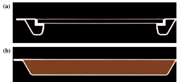
Figure 1. Cross-sections of the (a) ELEKTA Connexion Solid Inlay and (b) ELEKTA Connexion IGRT treatment couches with contoured couch structures.
