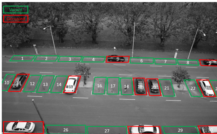
Figure 10.2: Image-based parking occupancy detection.
