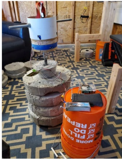
Figure 95. Static Load Testing of Coupling Release Mechanism.
