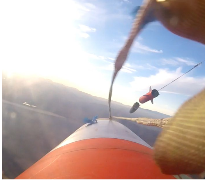
Figure 28. Premature Separation of Sled and Nosecone.
