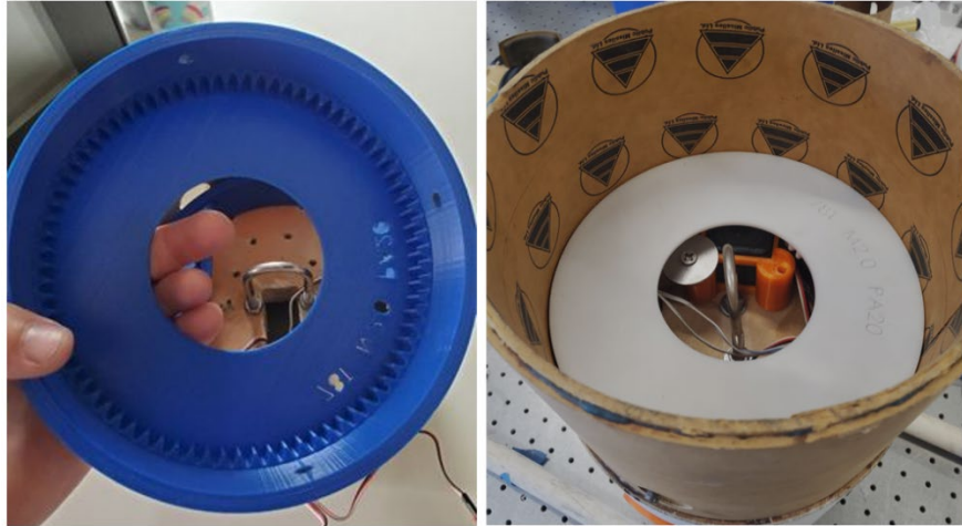
Figure 96. Planetary Gears with Details (Left) and as Installed (Right).
