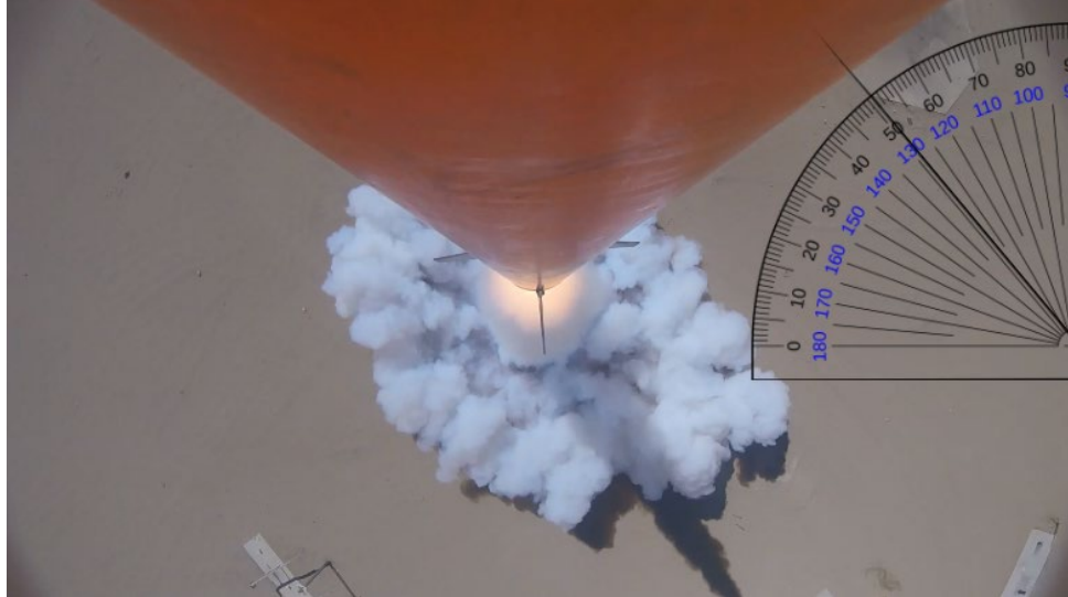
Figure 79. Reconstructing Rocket 5 Heading Data.
