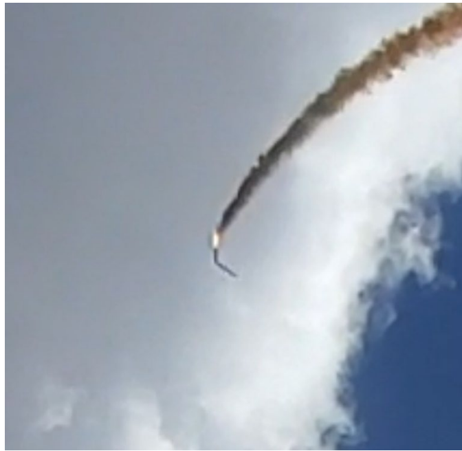
Figure 45. Rocket 2 Airframe Failure in Flight.
