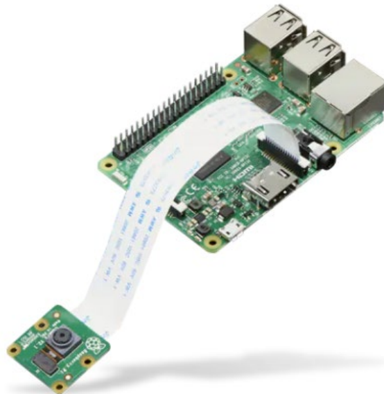
Figure 25. Raspberry Pi and V2 Camera. Adapted from [45].
