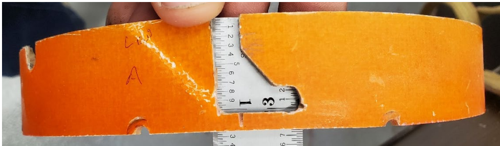
Figure 66. Damaged Sled Coupling Removed from Sled.
