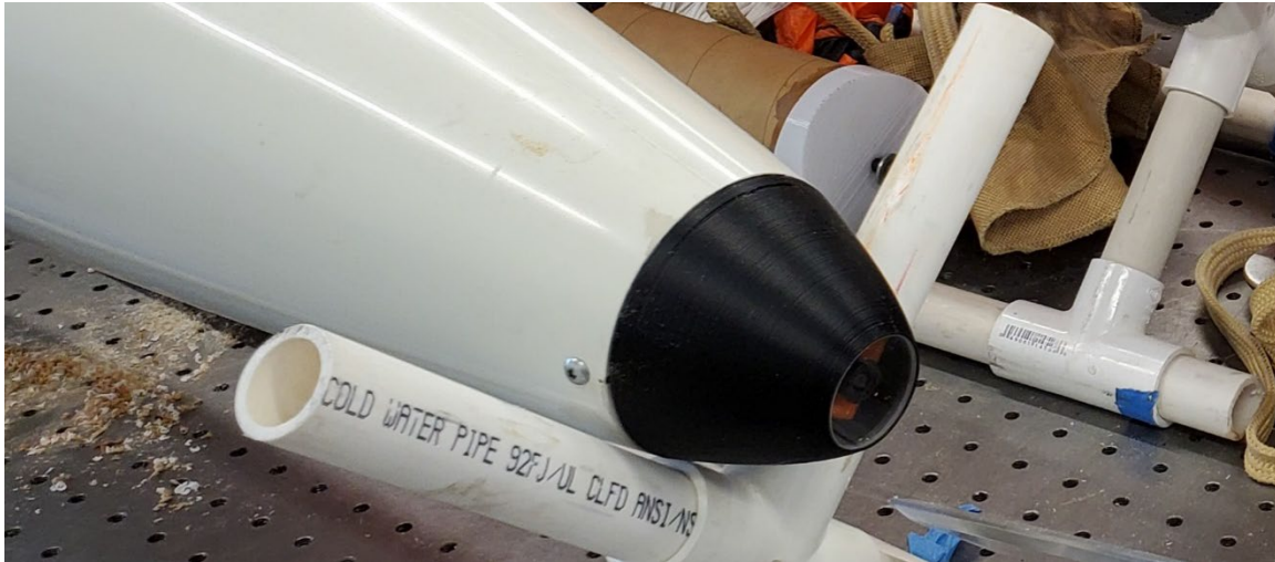
Figure 68. PETG with Carbon Nanotube Camera Housing.
