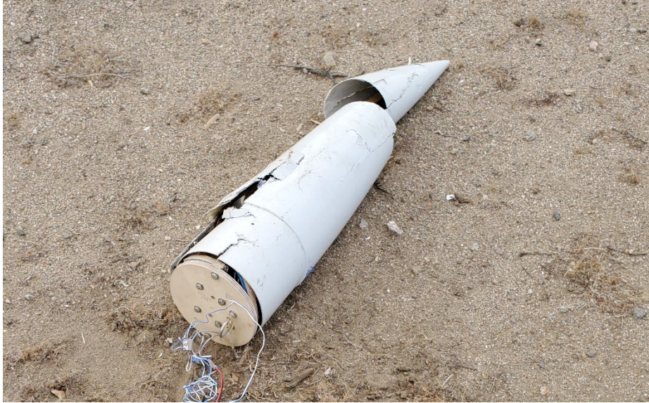
Figure 47. Rocket 2 Nosecone Following Impact with Ground.
