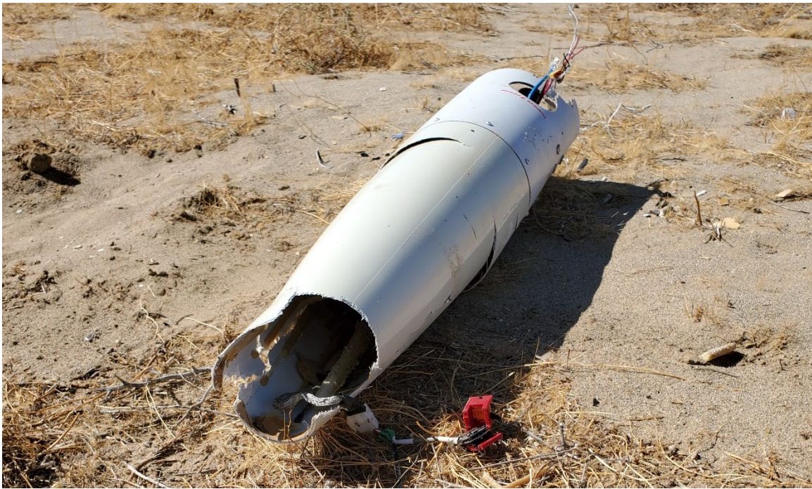
Figure 83. Rocket 5 Nosecone After Impact.
