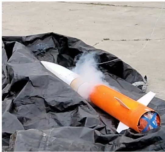
Figure 36. Ground Testing Sled Coupling Separation with 6 Shear Pins.
