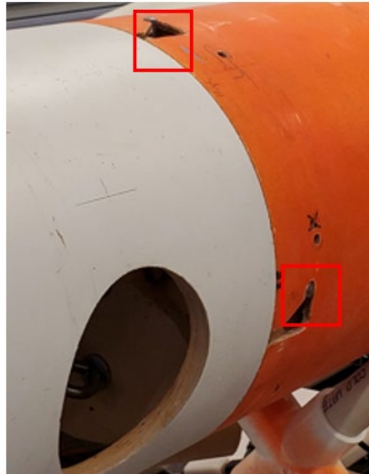
Figure 56. Airframe Cutouts for Pin Interlock Engagement.
