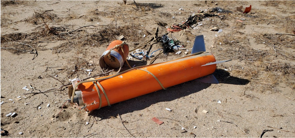
Figure 78. Rocket 5 Booster After Hard Landing.
