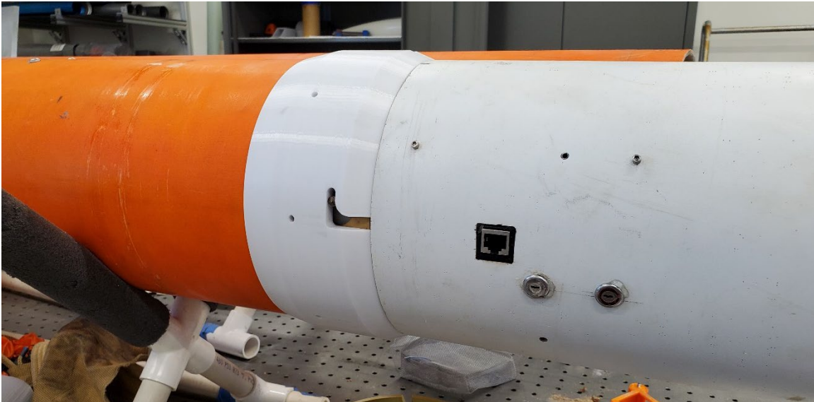
Figure 67. Polycarbonate Coupling Installed on Sled.
