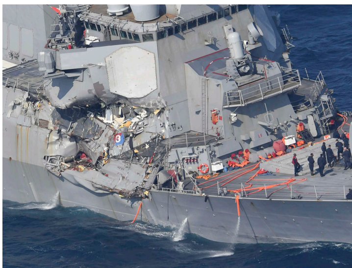
Figure 1. Damage from the USS Fitzgerald Collision with ACX Crystal Container Ship. Source: USNI (2017).
