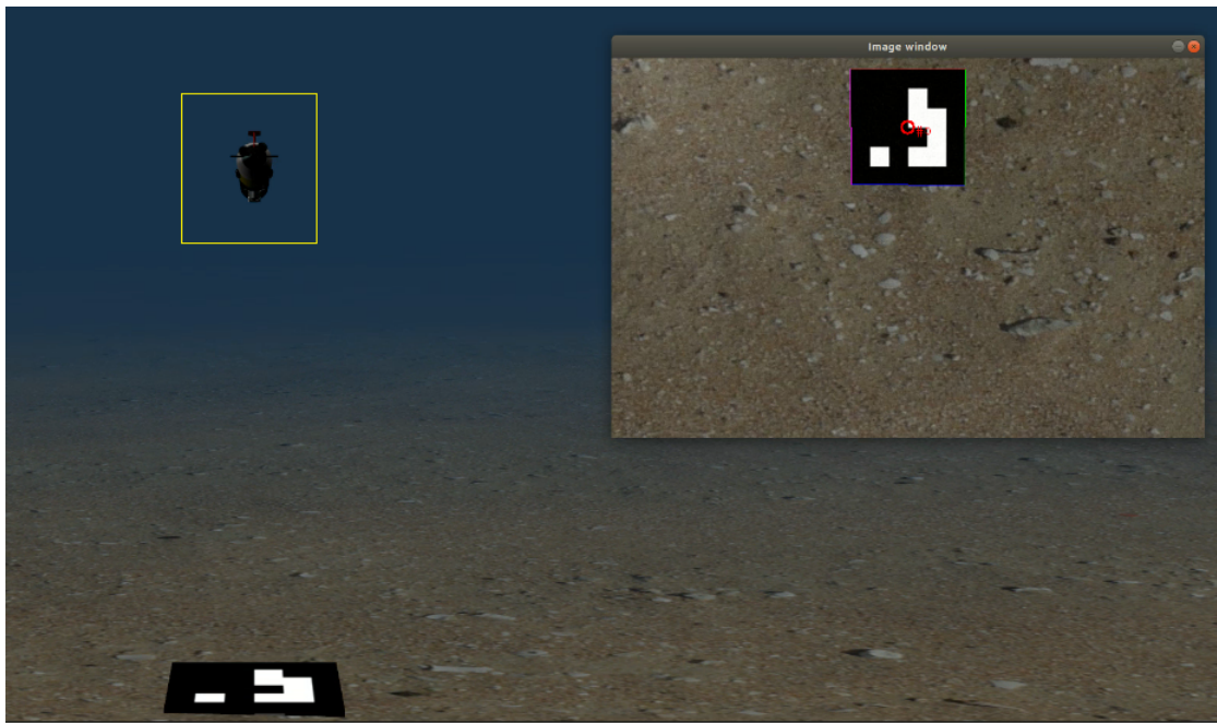
Image capture of AprilTag identification showing the spatial relationship between the vehicle and the AprilTag as well as the onboard camera image.
