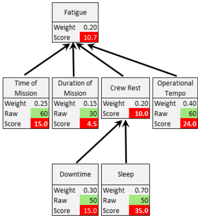
Figure 4. Seed model excerpt indicating subfactor weights, raw scores, and weighted scores for use in weighted score calculation demonstration
