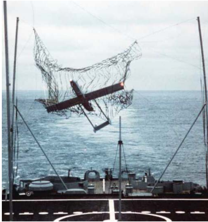
Figure 39. An RQ-2B Recovery Method on Navy Ships 683
