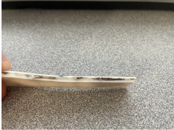
Figure 36. Low-quality print with PC blend and Electrifi.
