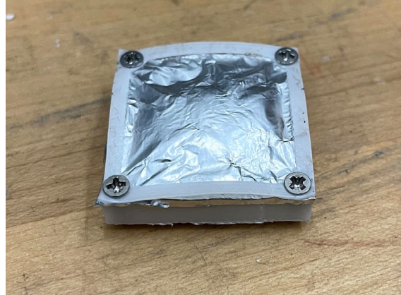
Figure 46. BN nanotube filled. The sample holder is made of PC and aluminum foil.
