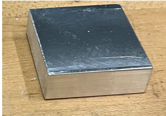
Figure 44. 2x Solid Aluminum block used as reference material in thermal testing
