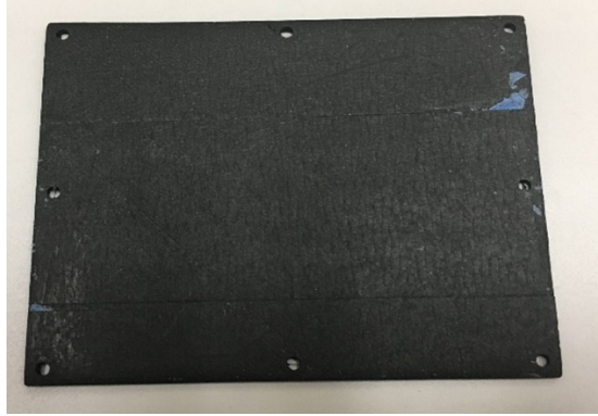
Figure 40. 3D-printed lid printed with CarbonX PA6+CF [Gen3].
