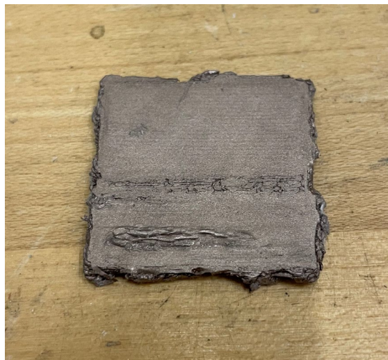
Figure 50. Commercial Electrifi with PCL/Copper.
