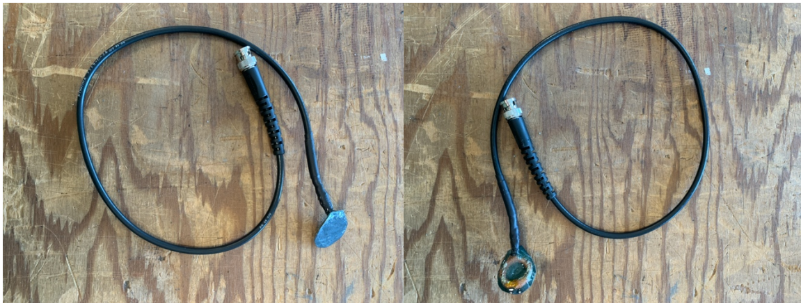
Figure 13. Photograph of top and bottom view of the magnetic field injector probe
