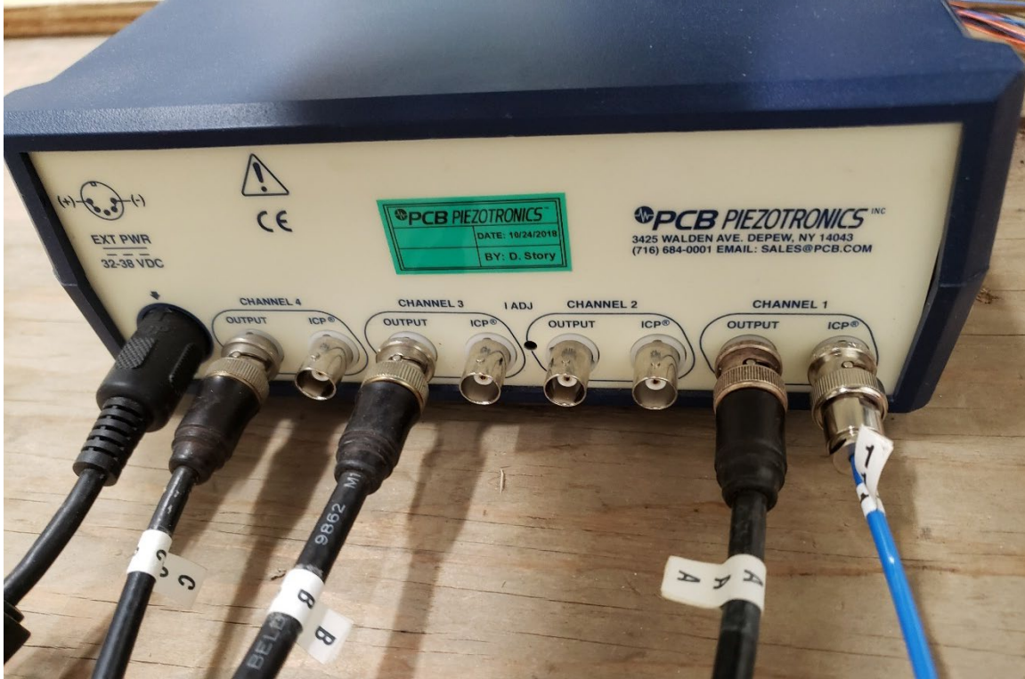
Figure 98. Proper BNC and ICP® sensor connection to signal conditioner for Channel 1
