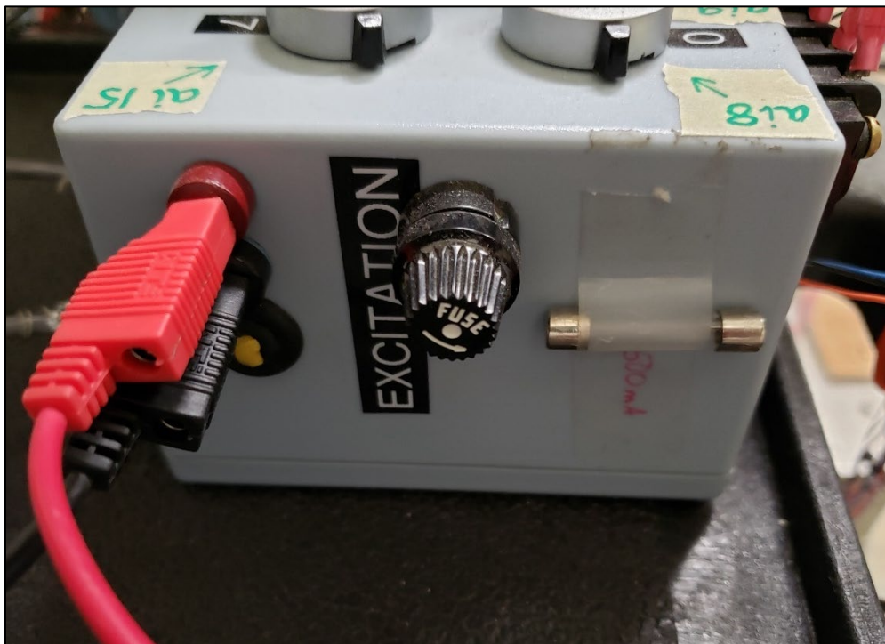
Figure 90. Correct banana plug connections from power supply to Wheatstone bridge
