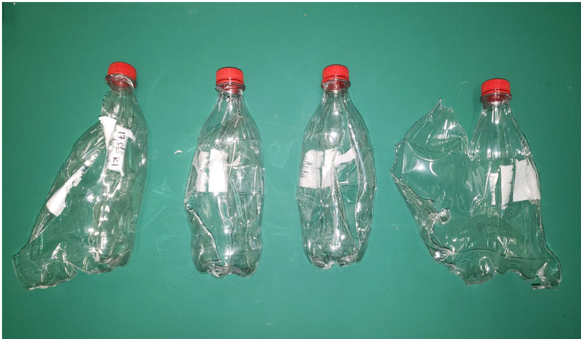
Figure 50. Recovered failed pressure vessels from pressure characterization testing
