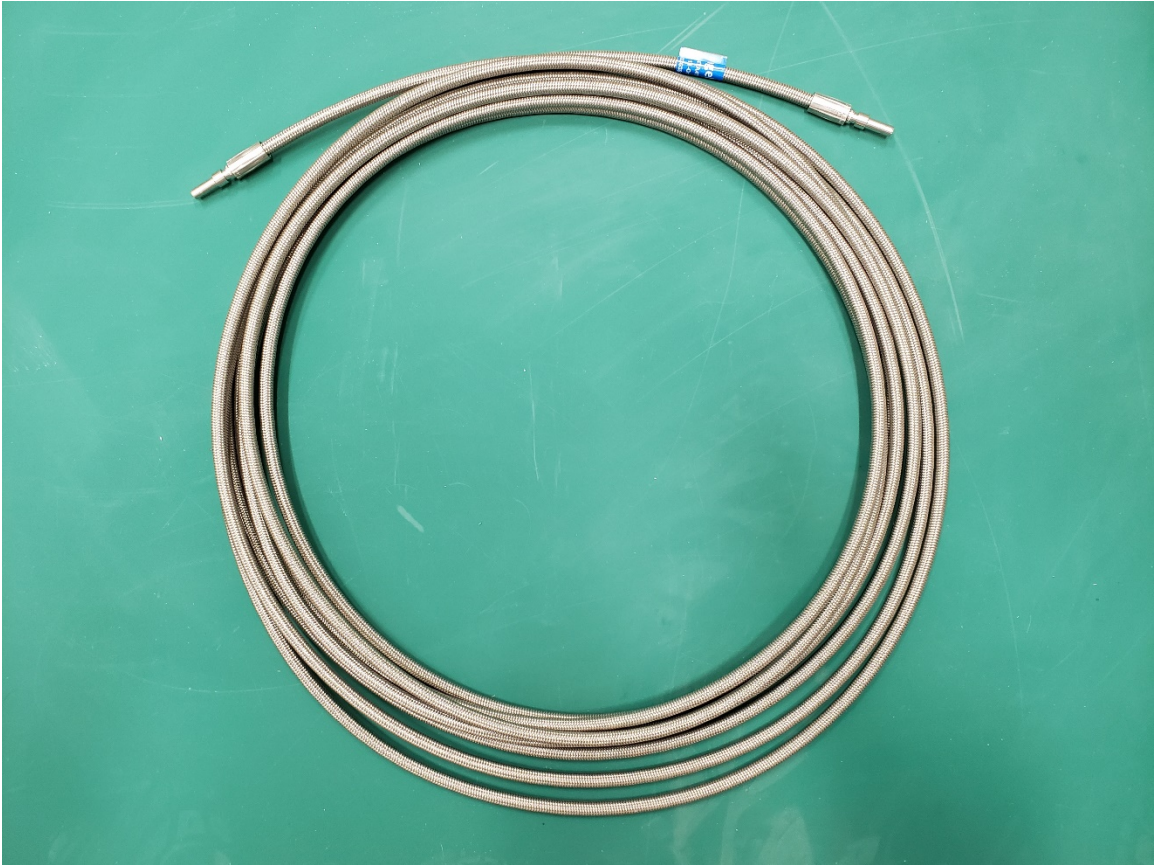
Figure 35. Flexible hose for out of water to in-water connection for testing
