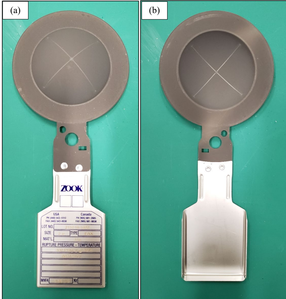
Figure 44. Non-fragmenting stainless-steel rupture disk: (a) inlet side (b) outlet side
