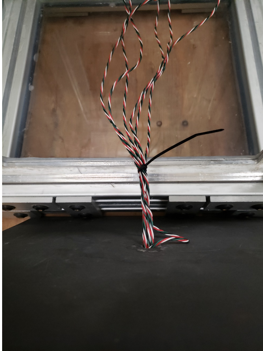
Figure 105. Zip-tie placement to prevent strain gage damage
