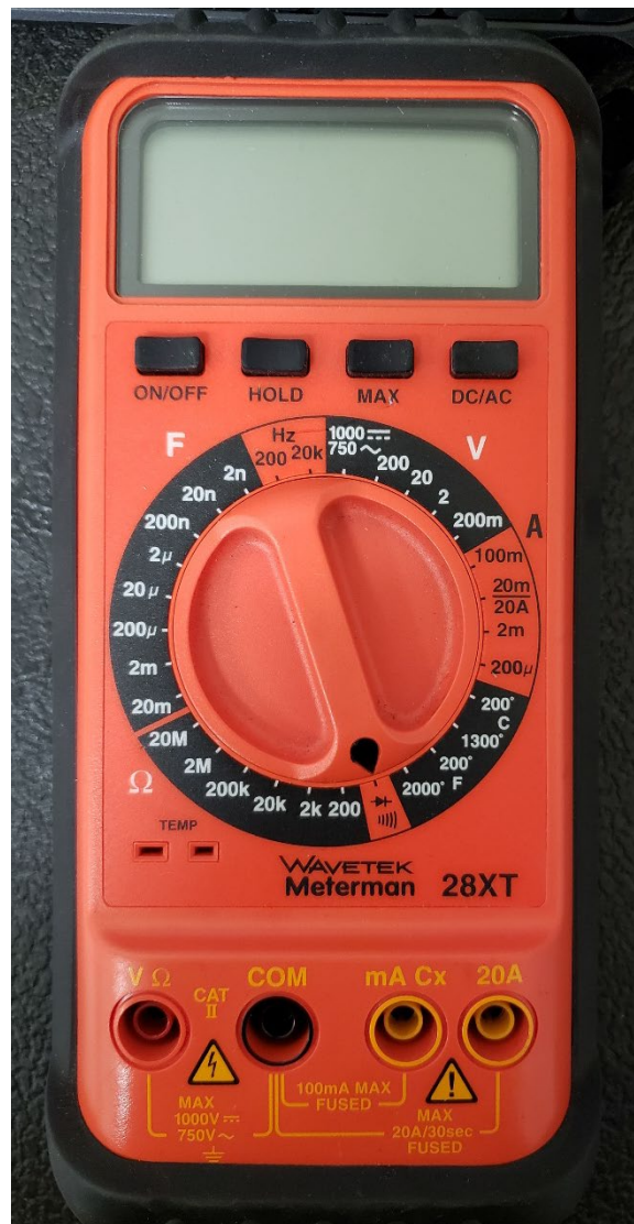
Figure 92. Continuity check function selected on DMM
