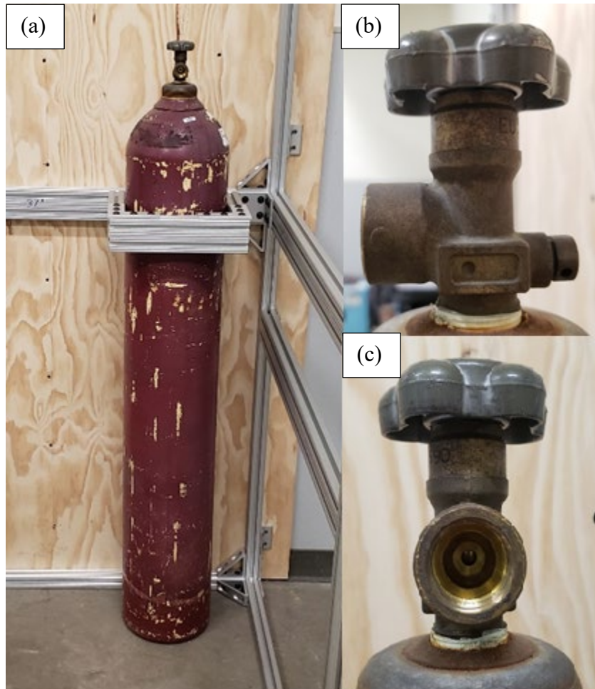
Figure 28. (a) Installed K-type industrial air compressed tank, (b) CGA-590 connection fitting, side-view, (c) CGA-590 connection fitting, front view (brass material)
