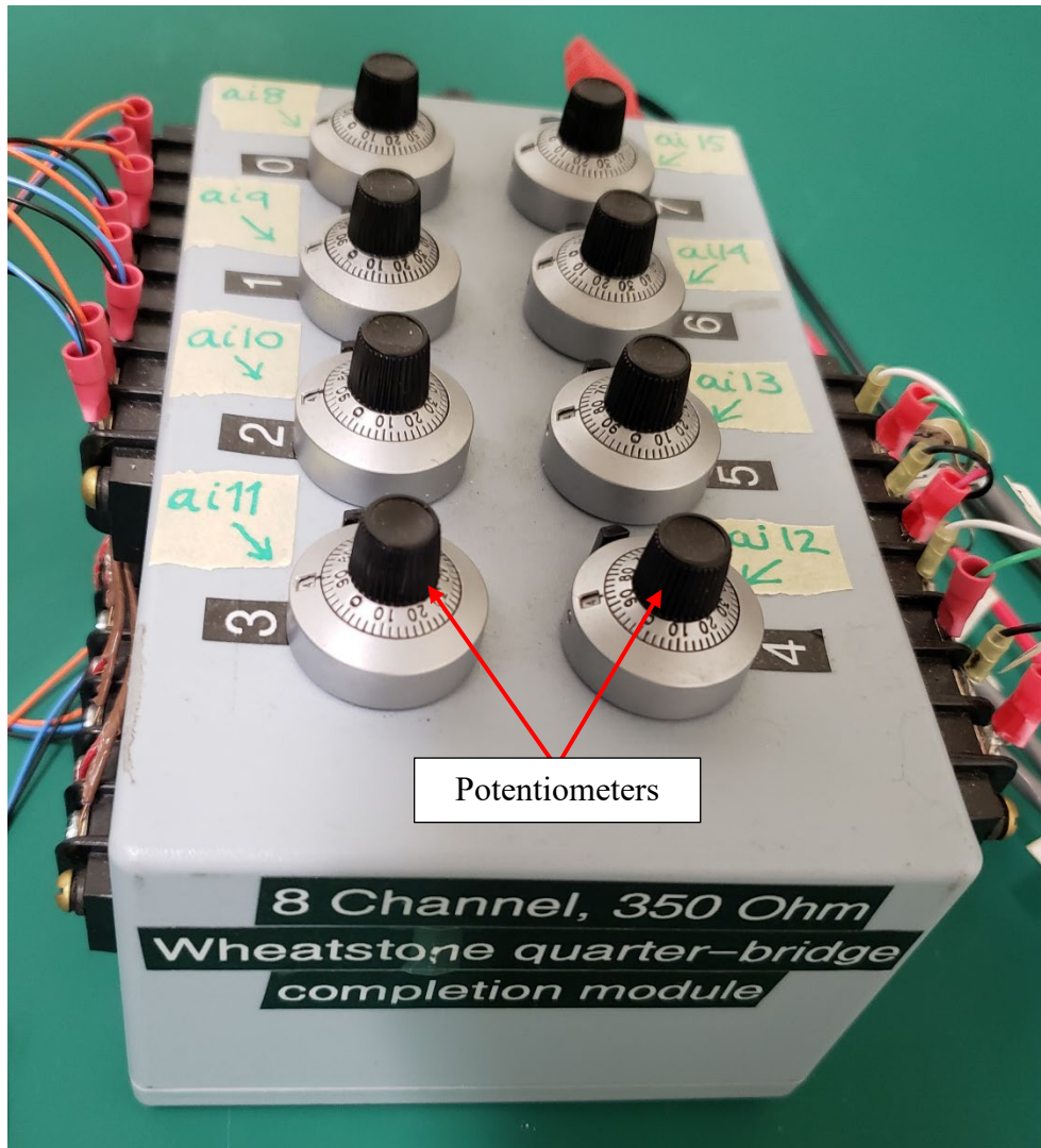
Figure 18. Wheatstone bridge with potentiometers
