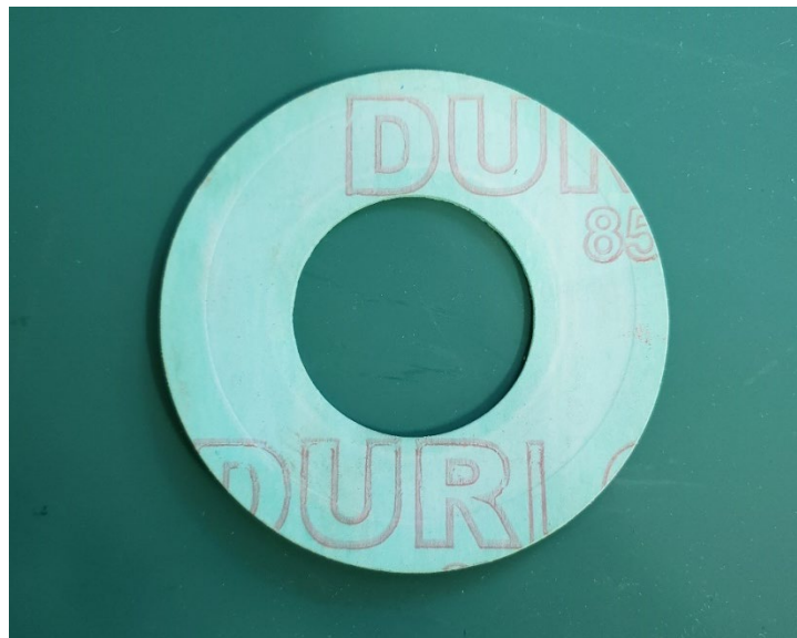
Figure 101. Gasket used for flange to holder sealing for CASPUR
