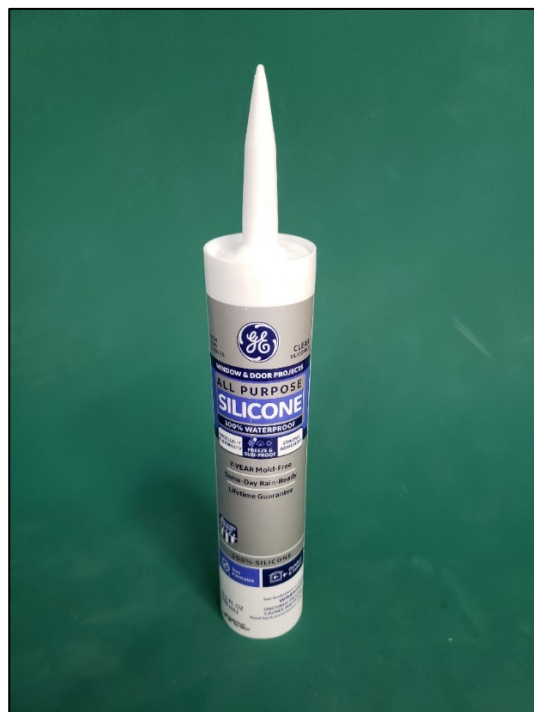
Figure 6. Waterproof sealant used to ensure AB backing condition
