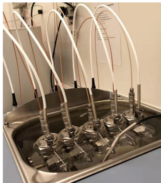
Figure 3. KHI test equipment showing the steel rocking cells placed in a cooling bath.
