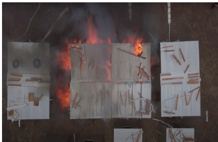
Figure 1. Large scale experiment performed via the IRIS-Fire project [2] in 2018 emphasizing the size of the external plume from vertical openings (doors and window) and leakage at joints of walls and roofs.
