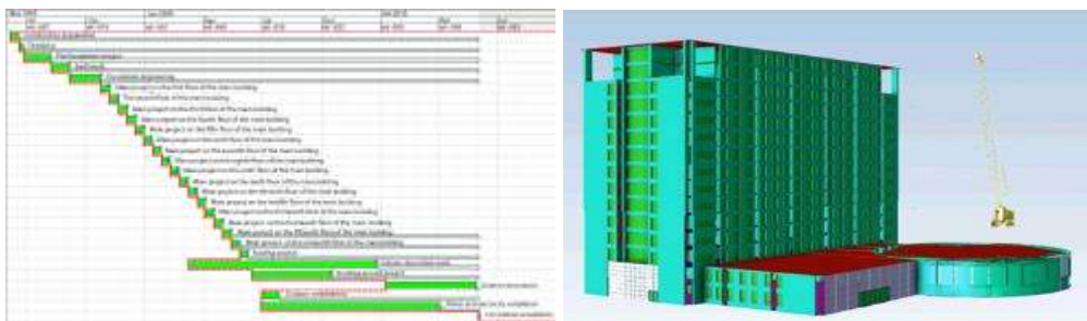
Figure 7: Construction progress and BIM model simulation of the main building.
