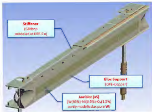
Figure 2: Mechanical layout of a tertiary TCT collimator jaw [5]. The main component i.e. the tungsten-based insert, composed by five jaw blocks, the copper block support and the copper based stiffener are shown.
