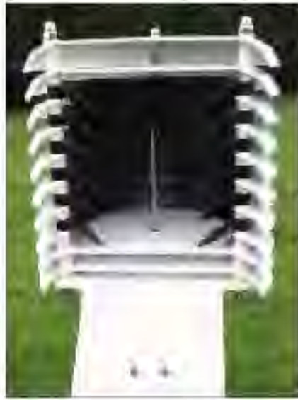
Figure 1: Cross-sectional view of a Stevenson Screen (Campbell, 2010)
