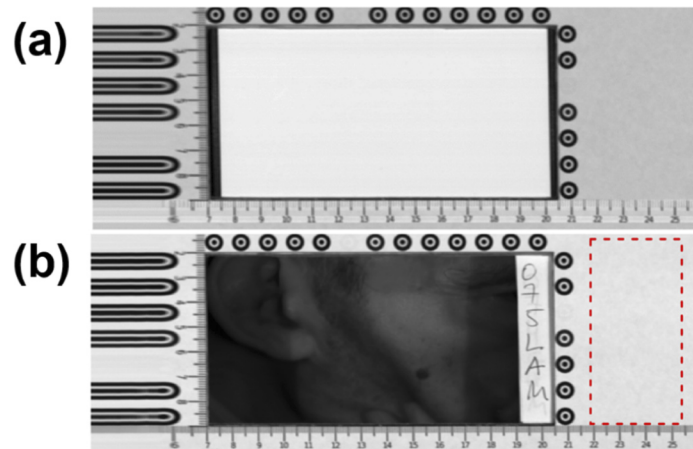
Fig. 2. The marker board used for the calibration and correction of the hyperspectral images. (a) Spectralon reflectance pattern. (b) Region (marked in red) used to obtain reflectance values for all 270 bands of the camera
