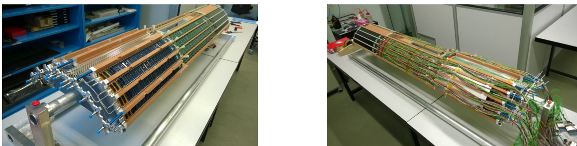
Figure 35. BPIX service half-cylinder during assembly: mechanics with power boards and cooling loops installed (left), and fully equipped BPIX service half-cylinder (right).
