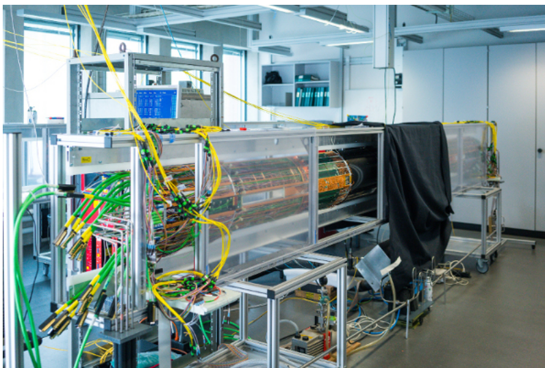
Figure 36. One half of the BPIX detector with the service half-cylinders connected. The detector system is placed on a rail system inside a 5 m long custom-built transport box.
