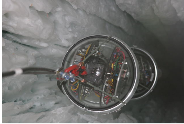
Figure 3.3: The Bubble Camera assembly goes down hole 57. The picture shows the two spheres.[IceCube wiki page: "Bubble Camera", https://wiki.icecube.wisc.edu/index.php/Bubble_Camera ].
