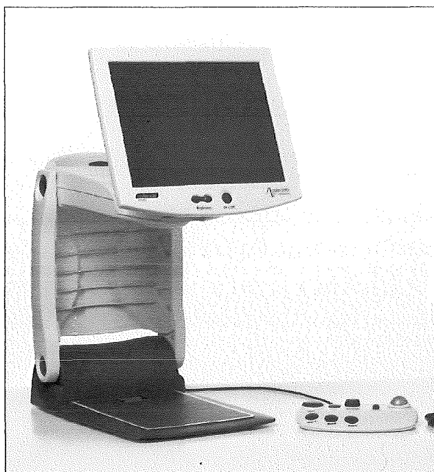
Figure 3.4: Prototype myReader low-vision reading aid with reader to the left and control panel to the right (from Pulse Data).
