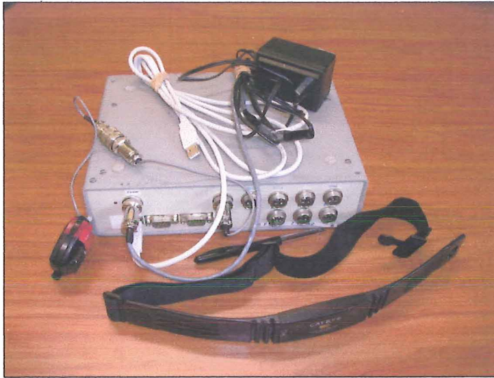
Figure 6.1: Modified polar sports heart-rate monitor, including chest strap, watch and signal processing hardware.
