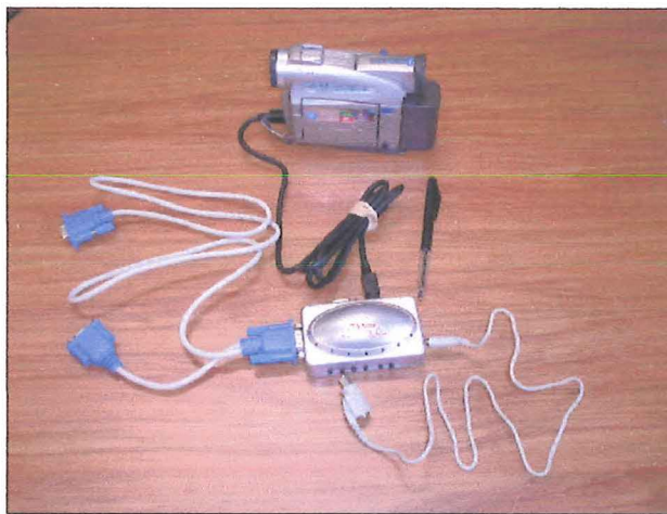
Figure 4.4: TV-PC converter used in to capture screen feed from monitor
