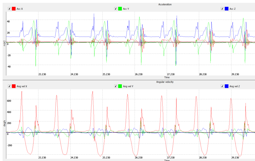
FIGURE 5.19: Forward walk's accelerometer and gyroscope signals
