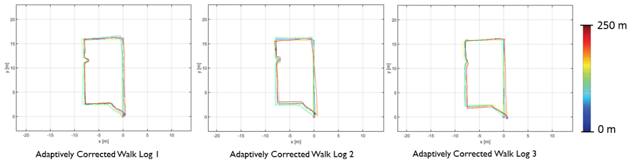
FIGURE 6.4: Adaptively Corrected Forward and Backward walk trajectories.
