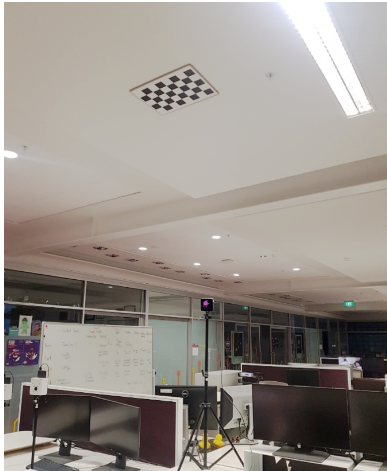
FIGURE 3.11: Ceiling mounted checkerboard used for the camera calibration
