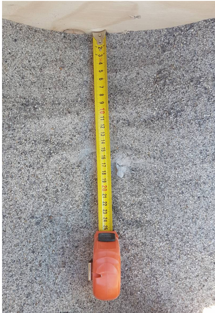
Figure 3.2: Results of bullet trap testing. The projectile penetrated roughly 190 mm into the sand.
