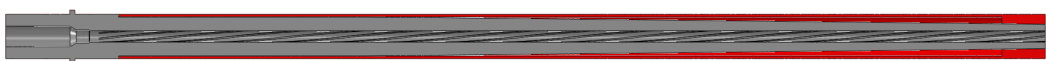
Figure 4.13: Depiction of barrel model in the sleeved configuration. Red represents the composite material.
