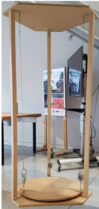
Figure 3.5: Trifilar pendulum used for measurement of center-of-mass location and mass moment of inertia.
