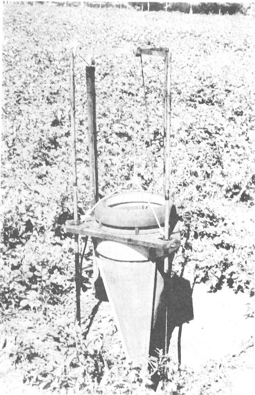
Plate 1. Johnson and Taylor suction trap showing the method of installation.
