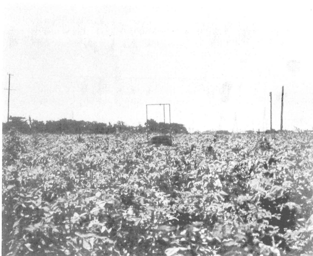
Plate 2. Johnson and Taylor suction trap in operating position with the induction fan level with the foliage cover.
