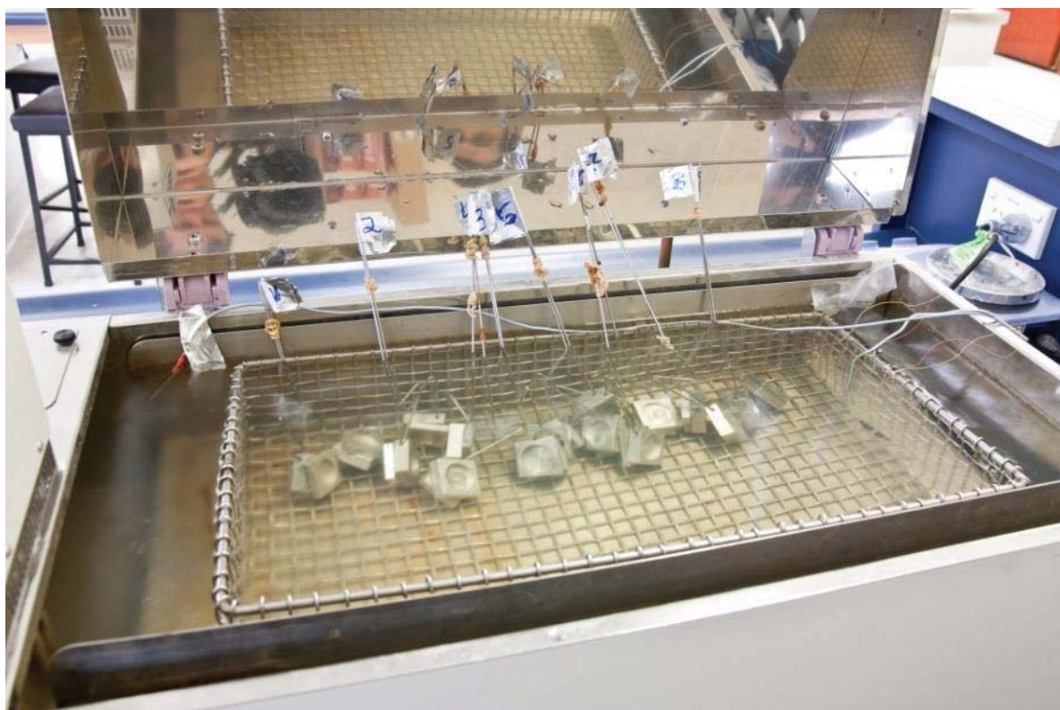
Figure B2. The aluminium cells during heating inside the water bath (Chapter 5)
