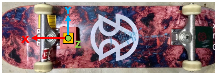
Figure 2 The placement of the instrumented device on the deck (rear view).
