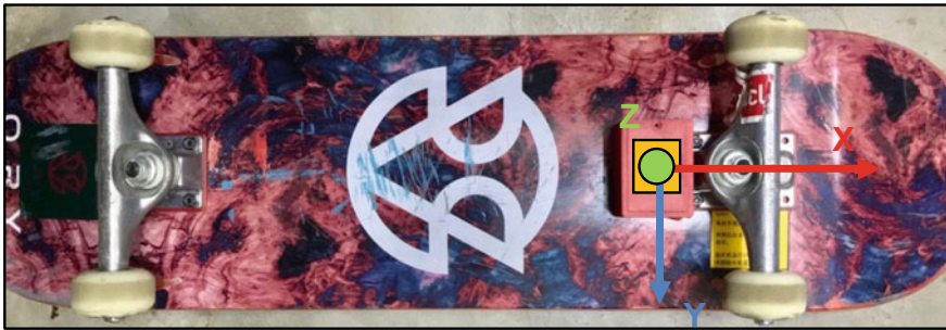
Fig. 2 Placement of the instrumented device on the skateboard
