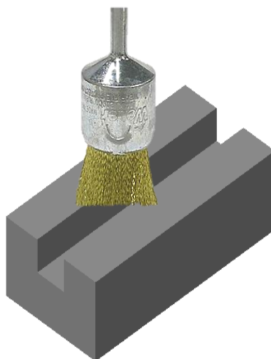
Figure 5. The deburring method proposed in the experiment, stainless steel end brush.
