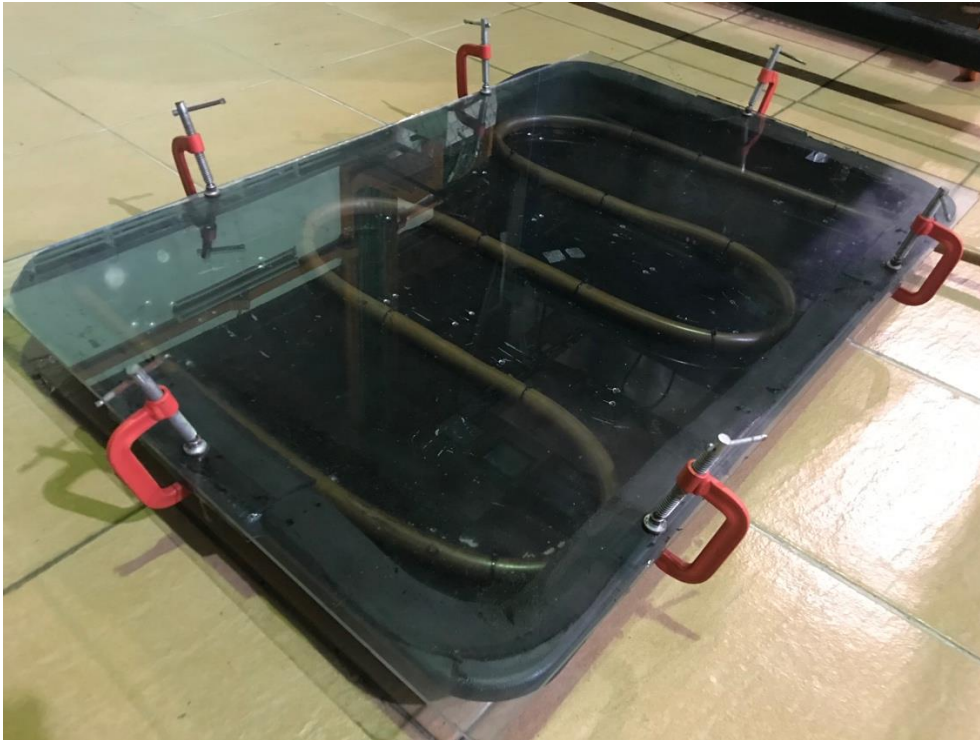
Fig. 1. Absorber collector with glass placed on top
