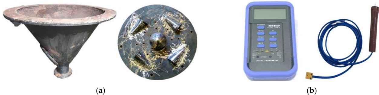
Figure 3. (a) Modification of hollow plate with four spoons and (b) digital thermometer and thermocouple for measurement data.
