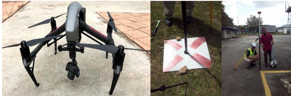
Figure 2. The photo of (a) multirotor drone (b) GCP marker (c) GCP measurement using GNSS receiver.
