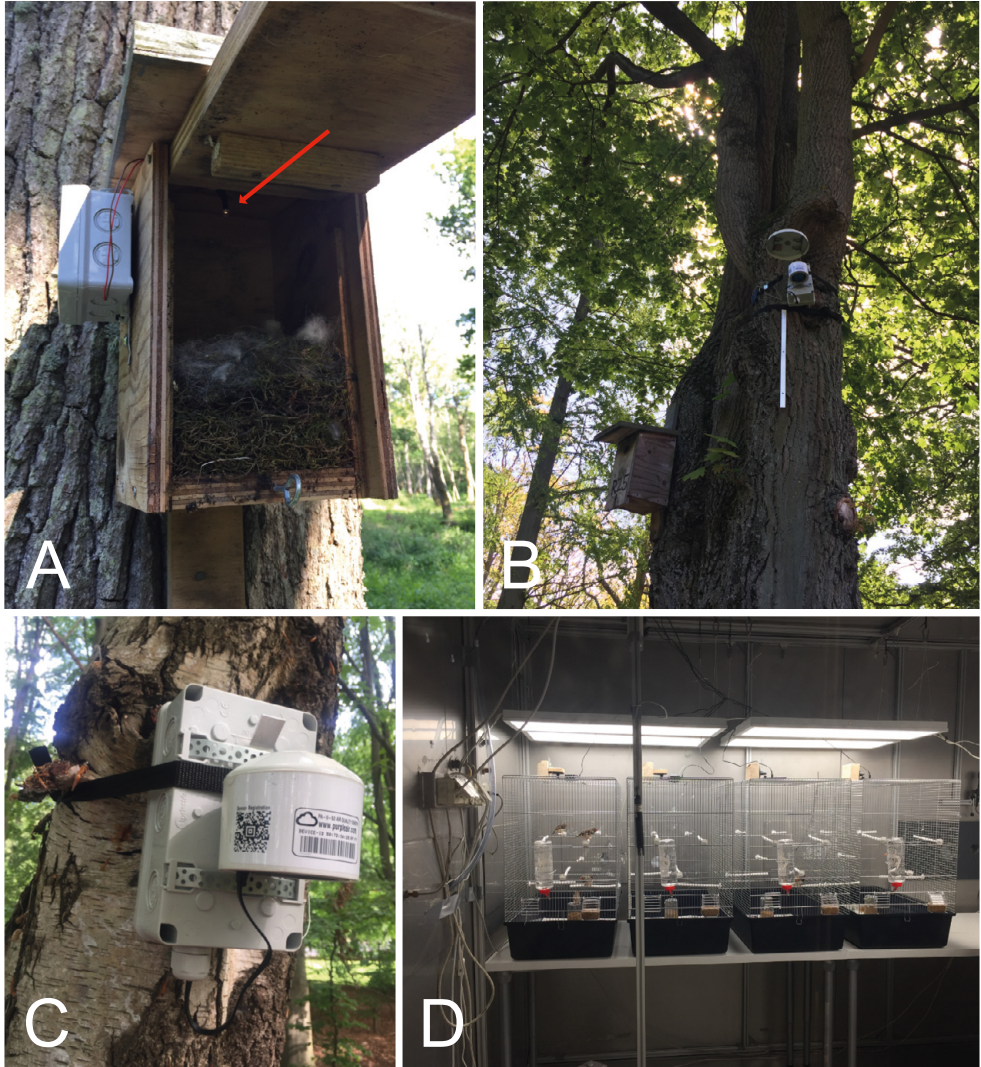
Figure 4. Representative pictures of different methods used. A) LED lamp emitting 3 lx, installed in a nest box of great tits. Red arrow indicates position of light source; paper II. B) NO 2 -diffusion sampler and PM-sensor installed on tree above nest box; paper V. C) Close-up of PM-sensor used in paper V. D) Picture inside exposure chamber used in papers I, III and IV.
