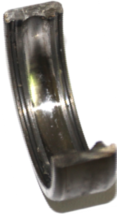
Figure 1. Outer ring defects
