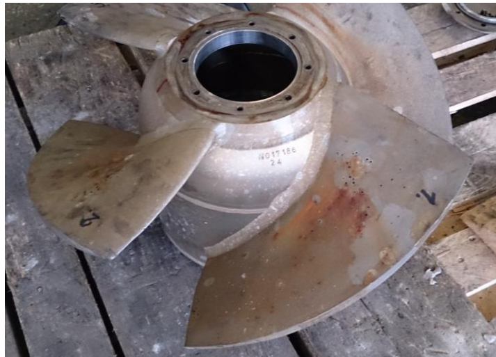
Figure 1. The damaged turbine blades
