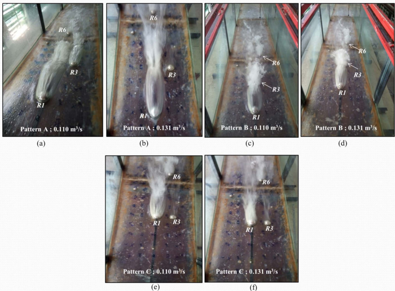
Figure 3. Experimental images: (a) pattern A, Q = 0.110 \text{ m}^3/\text{s} ; (b) pattern A, Q = 0.131 \text{ m}^3/\text{s} ; (c) pattern B, Q = 0.110 \text{ m}^3/\text{s} ; (d) pattern B, Q = 0.131 \text{ m}^3/\text{s} ; (e) pattern C, Q = 0.110 \text{ m}^3/\text{s} ; (f) pattern C, Q = 0.131 \text{ m}^3/\text{s} .
