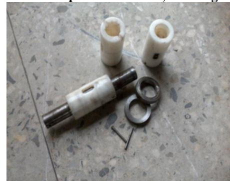
Fig 3. Metering device, shaft, bracer and pin
