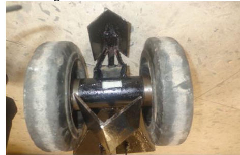
Fig 2. Furrow opener and closer, discharge spout
