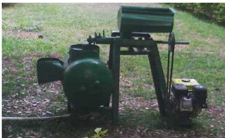
Figure 3: Fabricated locust beans seed dehulling machine
