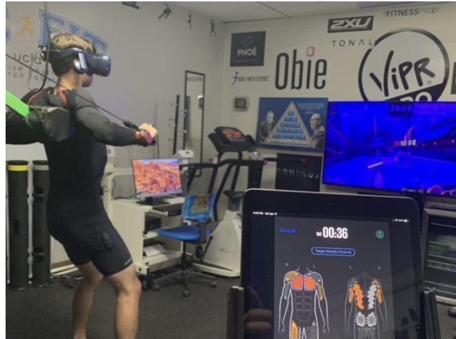
Figure 1. Participant donning the HMD and wrist-worn motion sensors during the IVR exergaming session while simultaneously being measured by an Athos compression suit embedded with an integrated sEMG measurement system. iPad displaying Athos app with real-time muscle activation via graduated shades of %MVIC (i.e., yellow to orange to red indicates low to moderate to high, respectively).
