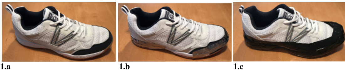
Figure 1. Preparation of experimental shoes. 1.a Indoor running shoe (Baseline) 1.b Lead tape added to fore and rear parts 1.c Concealed with the black tape
