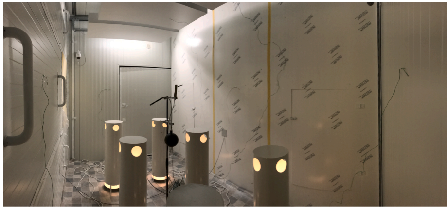
Fig. 8. Experimental measurement of PCM panels in a compensated chamber.
