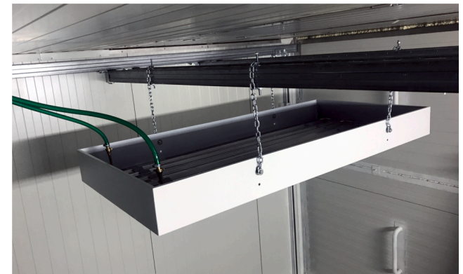
Fig. 4. The PCM-based cooling ceiling box prototype.
