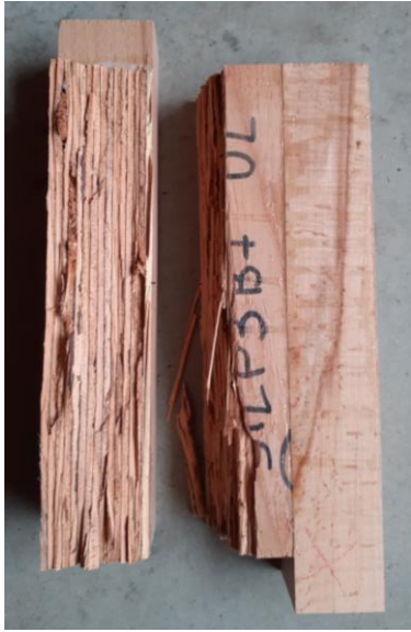
Figure 5: Parallel to the grain edgewise shear specimen failure
