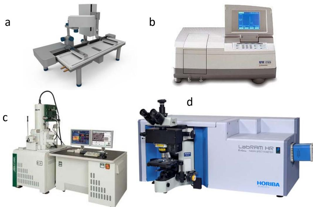
**Fig. 2.1** a) KSV NIMA LB mini-trough b) Shimadzu UV-1700 uv-vis spectrometer c) Jeol J-7100F Scanning Electron Microscope d) Jobin-Yvon Labram HR 800 Raman spectrometer. Images adapted from manufacturers
