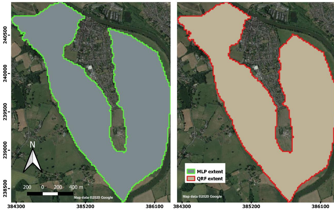
Figure 6.26: Predicted flood extent maps during flood peak - (a) MLP and (b) RF.
